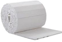
EPS 70 heat and sound insulation roll laminated with SAS hook and loop technology and pre-printed grid for easy laying of pipes. 28dB Impact noise reduction. Thermal Resistance 0.75m<sup>2</sup>K/W. Rolls are 1m x 12m.
