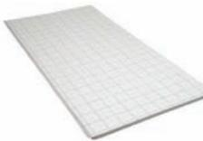
EPS 100 insulation slab with increased compressive strength for higher loadings. Laminated with SAS hook and loop technology and pre-printed grid for easy laying of pipes. Thermal Resistance 0.75m<sup>2</sup>K/W. Bi-folded slabs are 1m x 2m.
