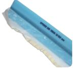
For use on solid screed floors as perimeter wall insulation, to reduce thermal bridging. Made of polyethylene with self adhesive backing and PE skirt providing tight seal between edge strip and insulation. Thermal resistance 0.22m<sup>2</sup>K/W. Supplied in 50m rolls, 150 x 10mm HxD.
